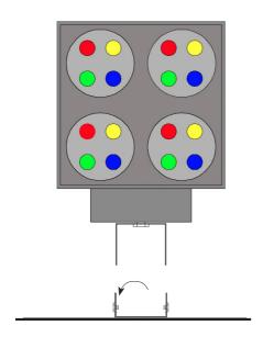
Fit fixture to the base and tighten screws evenly.
