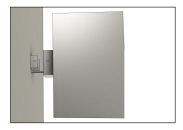
Fit fixture to the base and tighten screws evenly.
